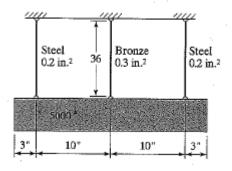
Taking moment about C,  $\Sigma M_C = 0$ : F1\*10-F3\*10 = 0 or F1=F3 (This can also be predicted from Symmetry of the bottom weight)
