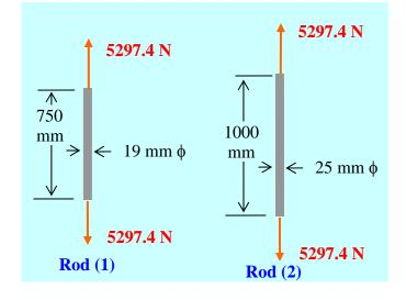
Then the axial deformation of rod (1) = (PL)/AE = (5297.4\*750)/(283.5\*206900) = 0.068 mm, and the axial deformation of rod (2) = (PL)/AE = (5297.4\*1000)/(490.9\*206900) = 0.052 mm
